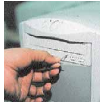
Open your jammed CD-ROM tray by inserting a pin in the front panel
